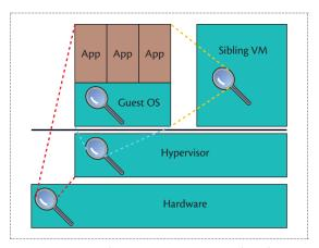
**Figure 1.** Monitor placement options in virtual machine introspection (VMI): in a sibling virtual machine (VM), the hypervisor, the guest OS, or the hardware. In-guest and hardware solutions require assistance from the hypervisor.
