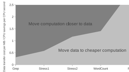
Fig. 1. Understanding when it makes sense to move the data: can the data transfer costs be made up by the CPU savings (due to different CPU costs on the source and destination node)? This figure plots the answer to this question as a function of their ratio. CPU intensive applications (Pi) are suitable to moving the data to cheaper cycles; data intensive applications (Grep) should move computation near data.
