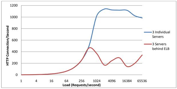
Figure 3b: Gain/Loss due to ELB in inter-zone setup (Servers without ELB vs. Servers with ELB)
