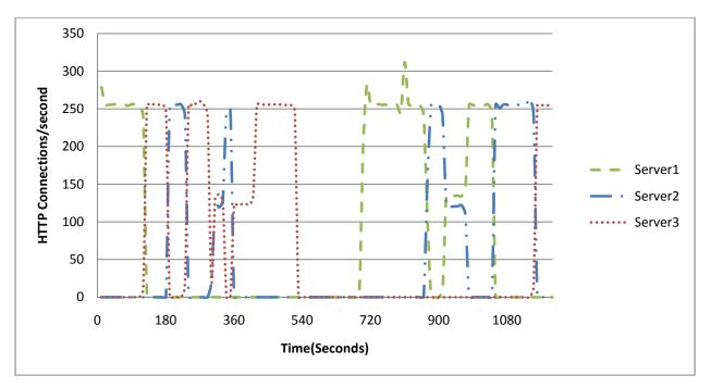
Figure 9: Result of convergence testing in inter-zone setup
