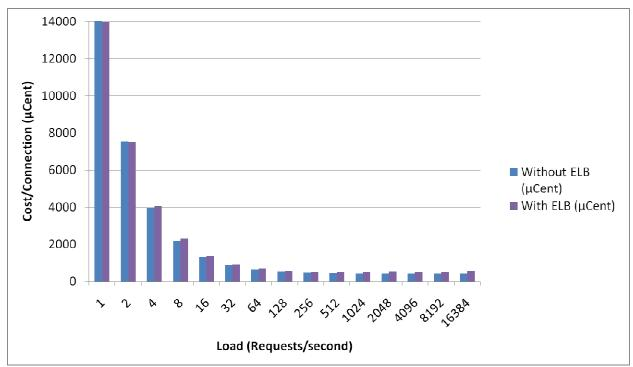
Figure 4b: Cost/connection in inter-zone setup
