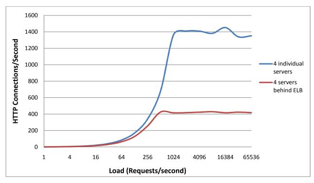
Figure 3a: Gain/Loss due to ELB in intra-zone setup (Indivudual Servers vs. ELB+Servers)
