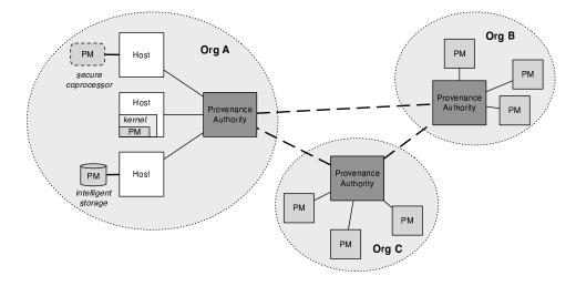
Figure 1: The proposed *end-to-end provenance system* (EEPS), a full-scale distributed provenance architecture, with provenance monitors (labeled PM) placed within the kernel and in trusted hardware. Provenance authorities negotiate cross-organization policy to ensure compliance.
