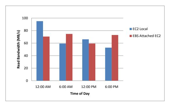
Figure 1: Sequential Read on Block Storage
