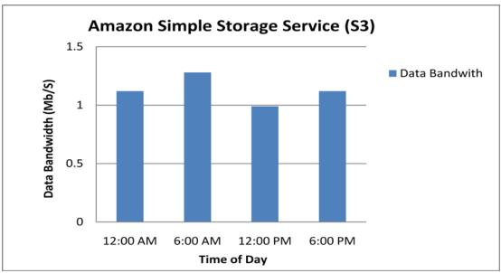
Figure 10: Data bandwidth on Amazon S3 (Stony Brook vantage point)
