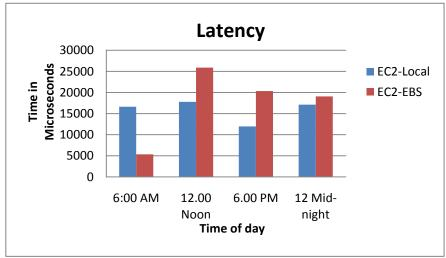
Figure 9: Write Latency for Amazon Block storage
