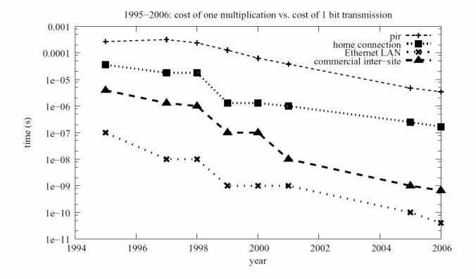
Comparison between the time required to perform PIR and the time taken to transfer the database, between 1995 and 2005. (logarithmic)
