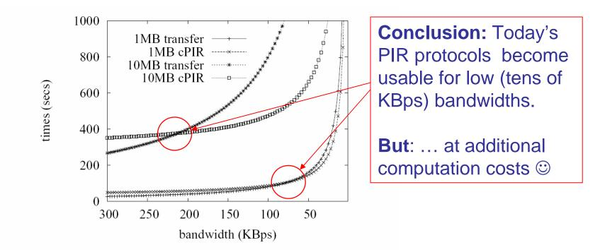
Low Bandwidth ( $t_{mul} < t_t$ , condition (4) does not hold): behavior of execution times for cPIR vs. database transfer times. If its (previously ignored) communication overheads are considered, the bandwidth thresholds below which cPIR becomes useful further decrease.
